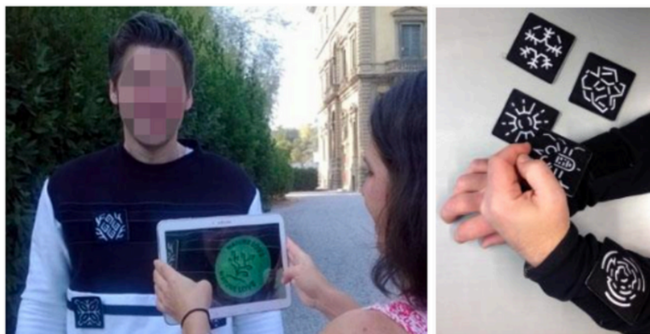
Figure 7. Using attachable visual markers for mobile AR interactions integrated into clothing (Häkkinen et al., 2021).
