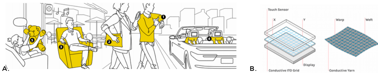
Figure 2. From Left to Right. a) Project Jacquard: Interactive digital textiles at scale, b) Textile structure is similar to that of multitouch capacitive panels used in tablets and mobile phones. Poupyrev, I., et al. (2016).
