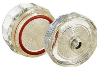
Figure 5.3: Membrane holder with 25 mm nominal diameter (from Whatman)
