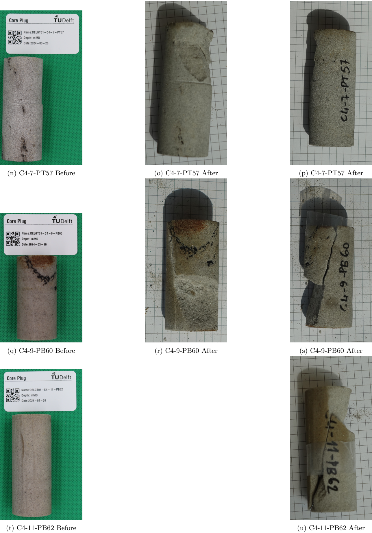
Figure 77: Samples that were tested on the UCS test, before and after.
