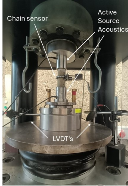
Figure 6: The set up of a UCS test.
