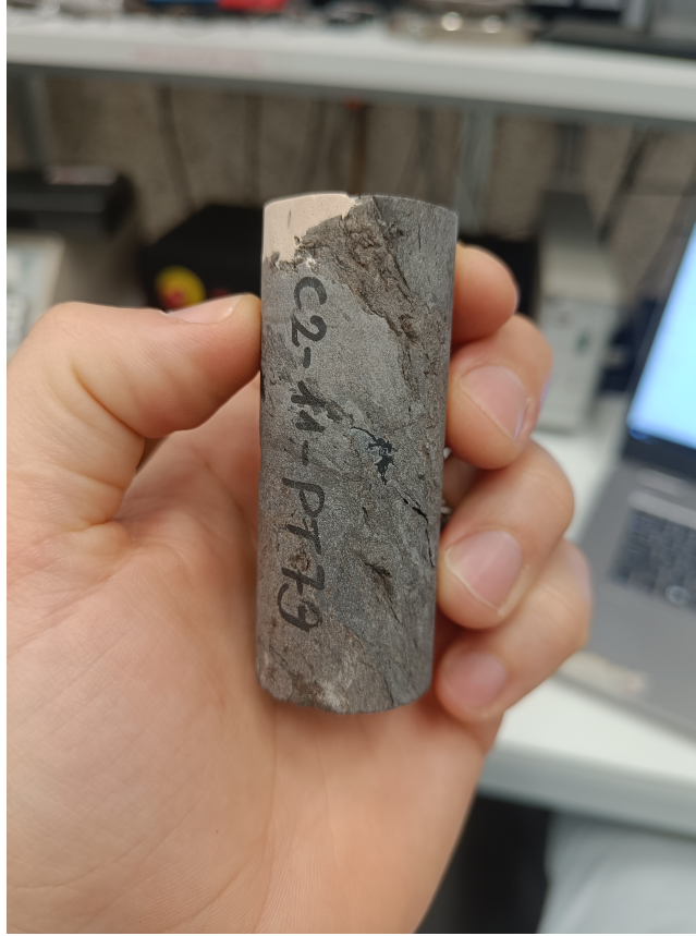
Figure 5: An example of a sample that has been repaired with gypsum in order to create two even surfaces on which pressure can be applied during the tests.
