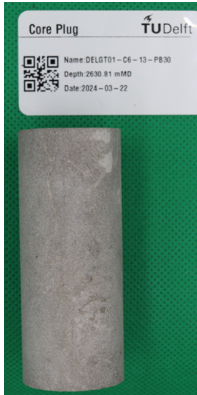
Figure 32: Sample C6 – 13 – PB30 , the sample that was more difficult to classify as sand or shale.
