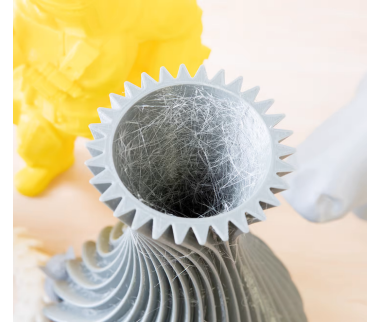
(c) Stringing is caused by unwanted oozing of the melt.
