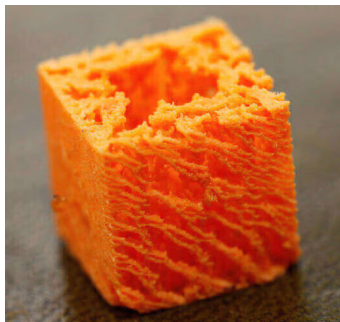
(a) Under-extrusion causes voids in the print.
