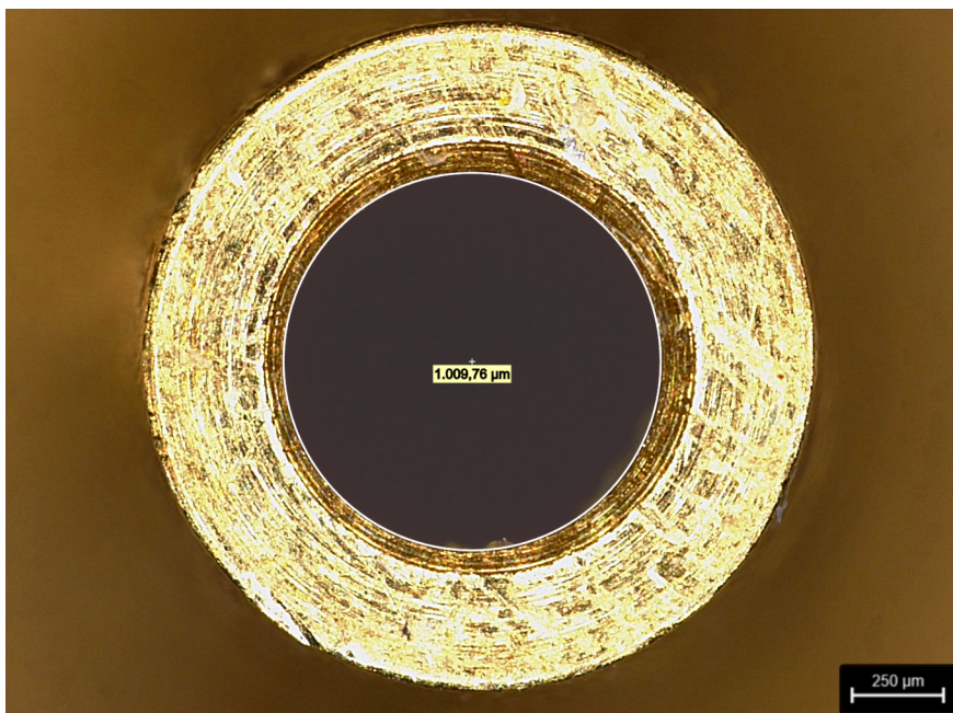
Figure 77: Example image of the opening of the guidance tube. A circle has been drawn to capture the diameter using the software provided by the digital microscope.
