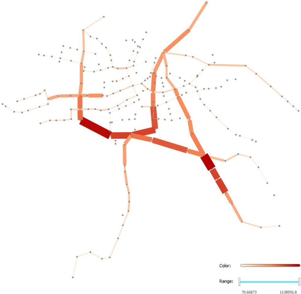
Figure 6 Link Criticality indicator (10-100%) for the links in the Amsterdam urban rail bound public transport network (thicker and more saturated red links indicate higher values)
