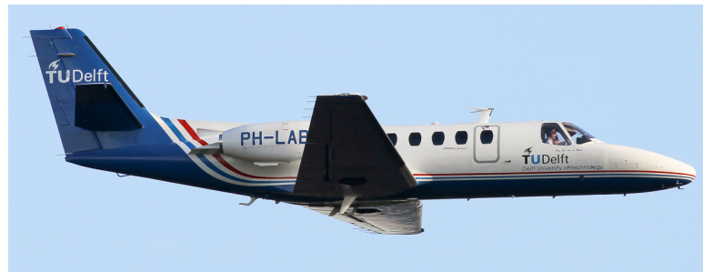
Figure 1.1: Cessna Citation PH-LAB research business jet aircraft operated by Delft University of Technology. Its fly-by-wire flight control system allows for the use of experimental flight controllers. 1
