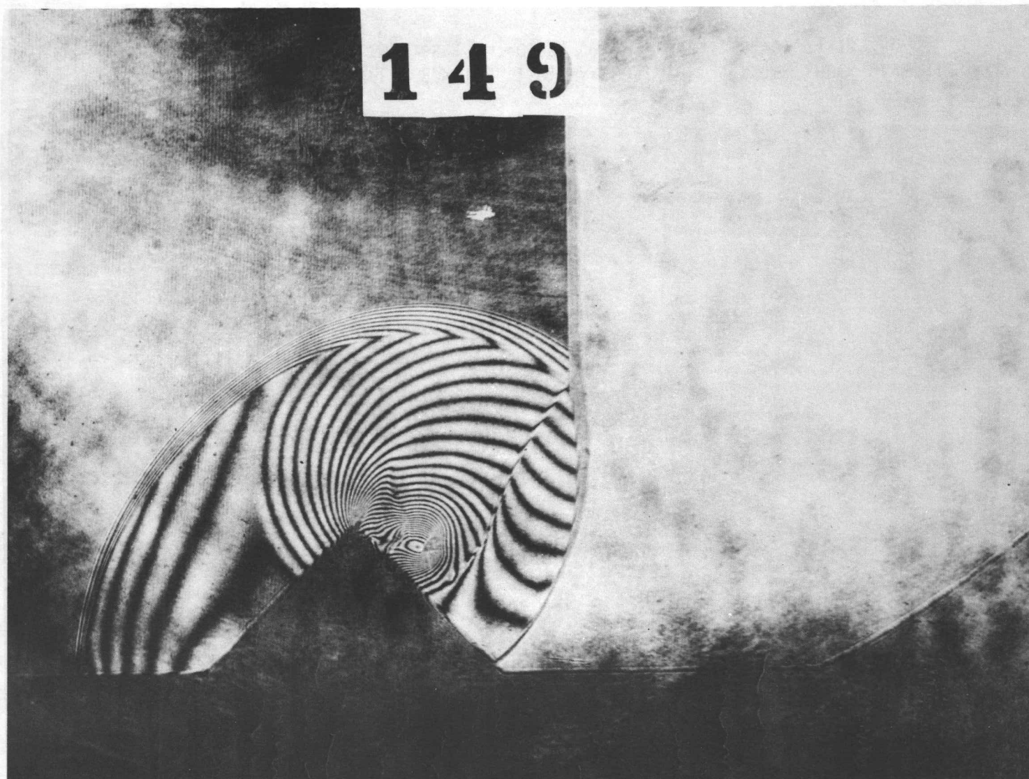
Fig. 18 INTERFEROGRAMS OF DIFFRACTION OF PLANAR SHOCK WAVE OVER A HALF - DIAMOND CYLINDER IN AIR FOR LONG - DURATION FLOWFIELD, M_S=1.60 , M_1=0.69 , SUBSONIC FLOW.
