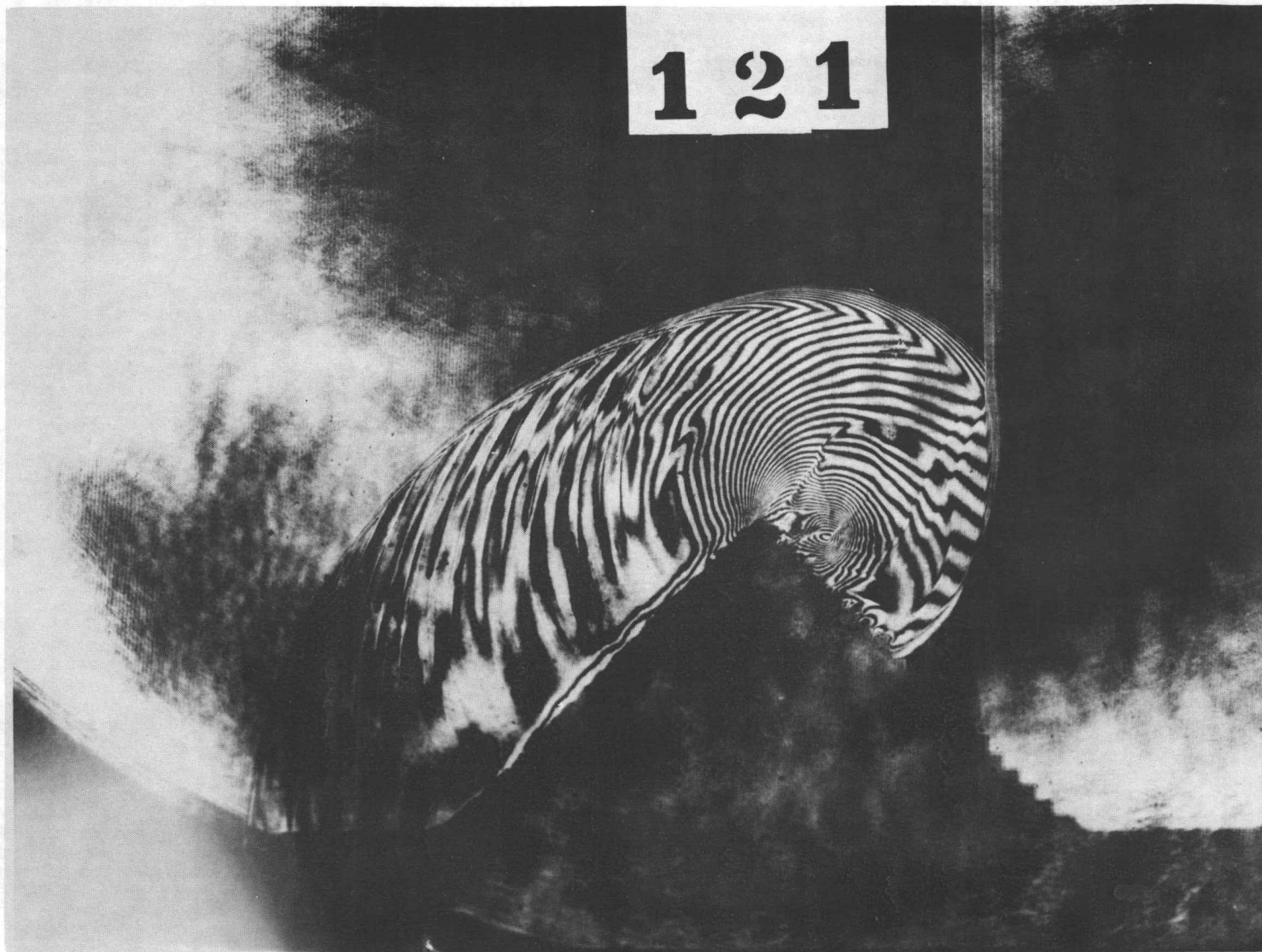
( b ) AN INTERFEROGRAM (No. 121) TAKEN AT 89 \mu\text{s} AFTER SHOCK WAVE HITS CORNER; M_s=1.59 , M_1=0.68 ; P_0=32.66\text{KPa} , \rho_0=38.30 \times 10^{-2}\text{kg/m}^3 , T_0=297.4^\circ\text{K}
