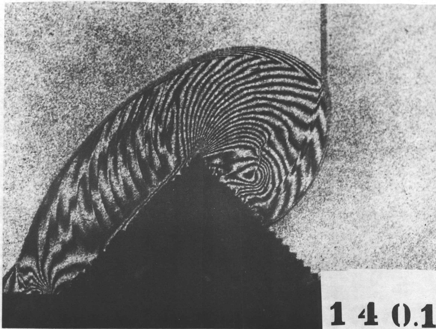
( d ) AN INTERFEROGRAM (No. 140.1) TAKEN AT 65 \mu\text{s} AFTER SHOCK WAVE HITS CORNER; M_s=2.44 , M_1=1.16 ; P_0=9.33\text{KPa} , \rho_0=10.97 \times 10^{-2}\text{kg/m}^3 , T_0=296.7^\circ\text{K}
