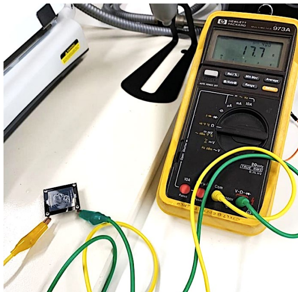
Figure 35 – Optical image of the conductivity measured across the Al/PDMS membrane.
