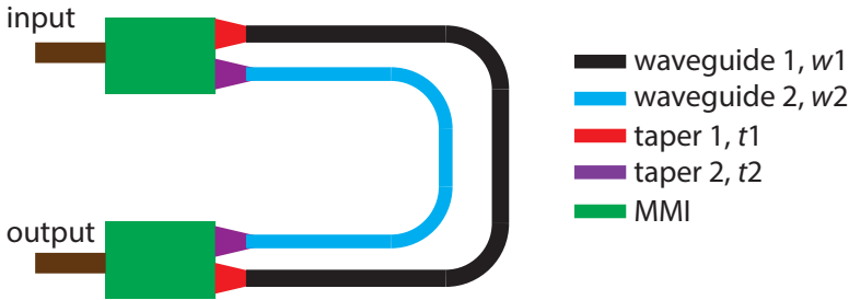
Figure 4.8: Schematic of the MZI design with two waveguide widths, giving an FSR robust to waveguide-width variations. The sketched MZI is shaped differently from the one in Figure 1.8, but is topologically the same.
