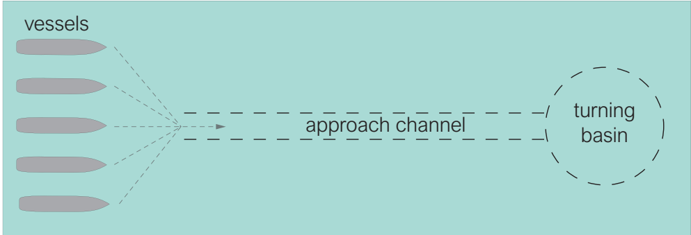
Figure 3.4: Port approach system considered as a service system in queueing theory (by TU Delft – Ports and Waterways is licenced under CC BY-NC-SA 4.0).
