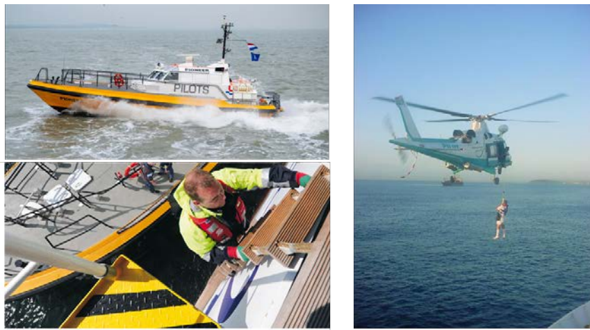
Figure 3.2: Pilot boarding; left: by boat and ladder ( Shipping pilot by www.pikist.com is licenced under CC0 1.0); right: Pilot boarding a vessel by helicopter (by Hokewiki is licenced under CC BY-SA 3.0).
