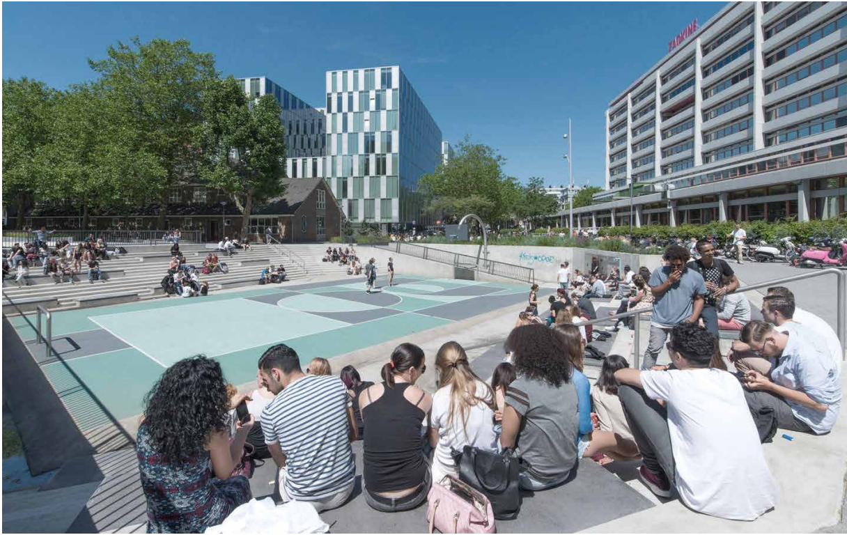
FIGURE 7.16 The Water Square Bentheplein in Rotterdam, the Netherlands, is designed as an urban public space that can also store storm water during extreme rainfall. Photo credit: Jeroen Musch.
