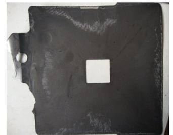
Figure 4-31 Carbon electrode used in PCCell MCDI stack
