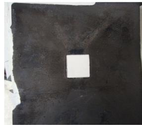
Figure 4-30 Carbon electrode used in Voltea MCDI stack
