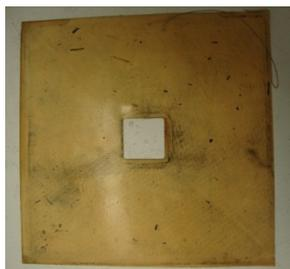
Figure 4-32 Used AEM PCCell MCDI stack
