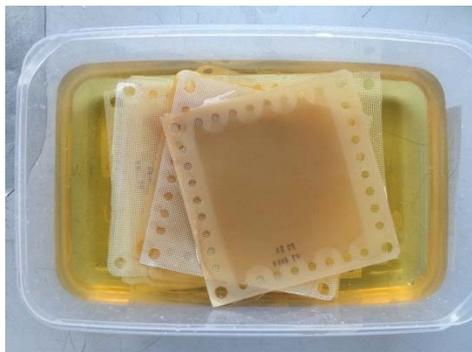
Figure 9-14 Soaking of the ED membranes in NaCl solution
