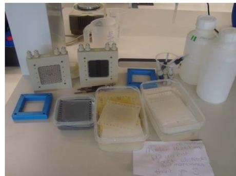
Figure 9-15 Disassembled ED stack
