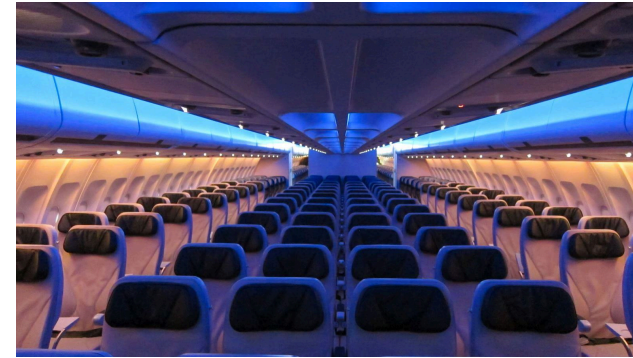
fig. 19 Ambient Lighting provides general lighting for the cabin
