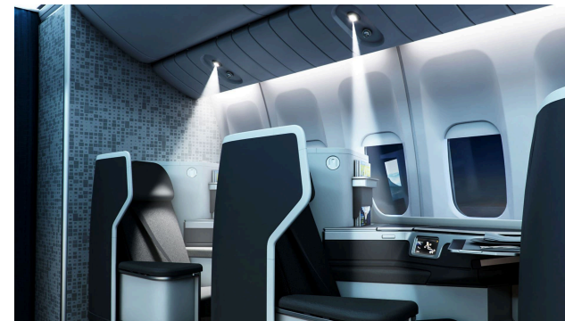
fig. 20 Task Lighting assists passengers with specific activities, such as reading or working.
