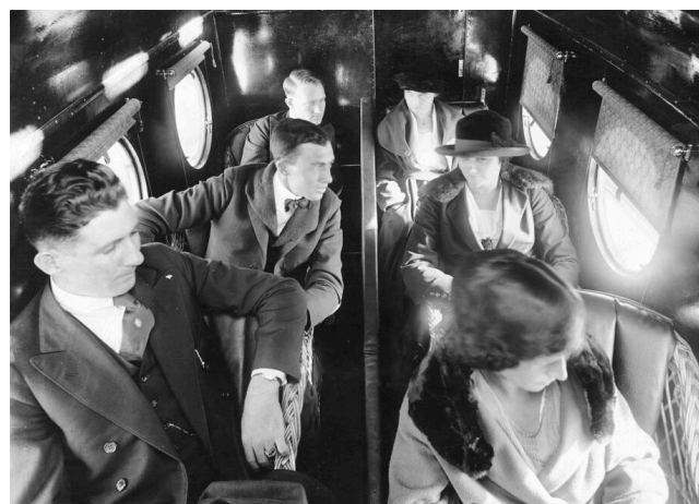
fig 9. The interior of an Aeromarine Airways airliner. Note the wicker seats. Aeromarine Airways flew for four years, from 1920-1924.
