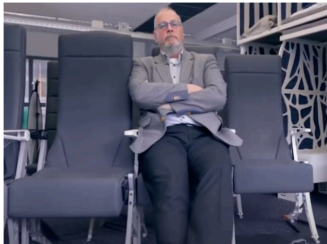
fig. 18 Peter Vink in the cabin design concept for TU Delft's Flying-V with a staggered seating line up.
