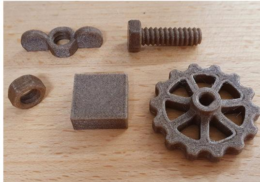
Figure 4.6: Successfully 3D printed samples using the MGS-1/PLA filament.
