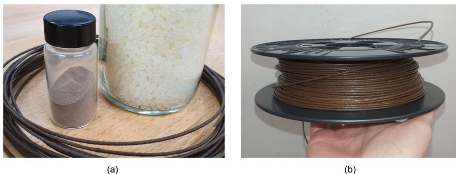
Figure 4.4: (a) Sieved MGS-1 particles and PLA pellets, and (b) the produced MGS-1/PLA composite filament.
