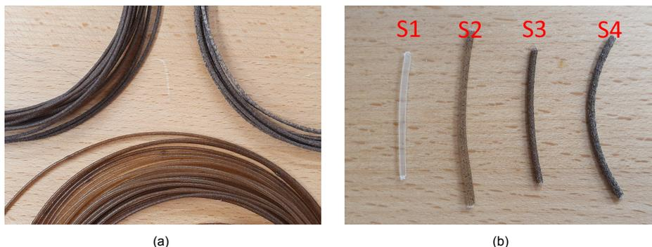
Figure 4.5: (a) Different concentrations of MGS-1 and PLA as derived by the color, and (b) filament strands with differing concentrations to measure the density, ranging from low (S1) to high (S4) MGS-1 weight fractions.
