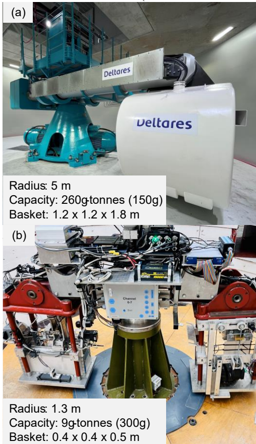
Figure 1) are the two key facilities adopted to investigate the lateral behaviour of monopiles in sand under monotonic and cyclic loading in the MIDAS project.
