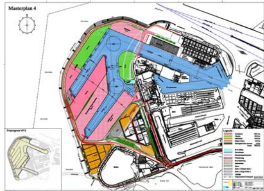
Figure 5-7. Latest design, with some minor changes in comparison with Masterplan 1, which increased the length of the quays (Port of Rotterdam, 2009)
