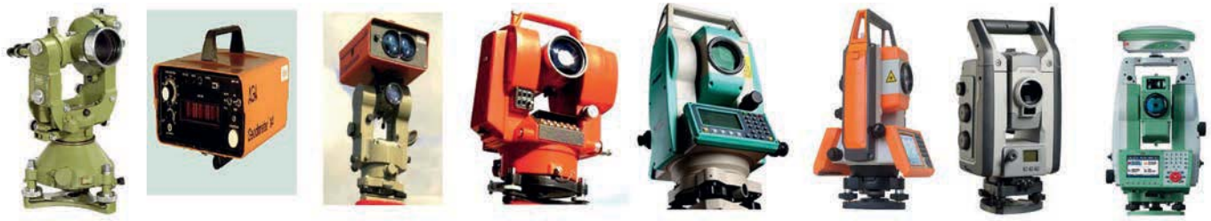
▲ Figure 3, Evolution from theodolite to today's total station.
