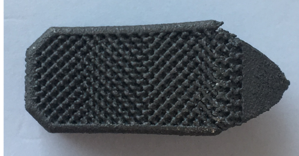
Figure 5.28: Top view of a tested spinal cage using a quasi-static compression test.
