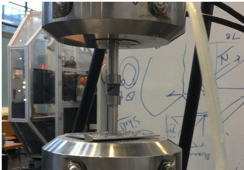
Figure 4.25: The set-up for fatigue tests.
