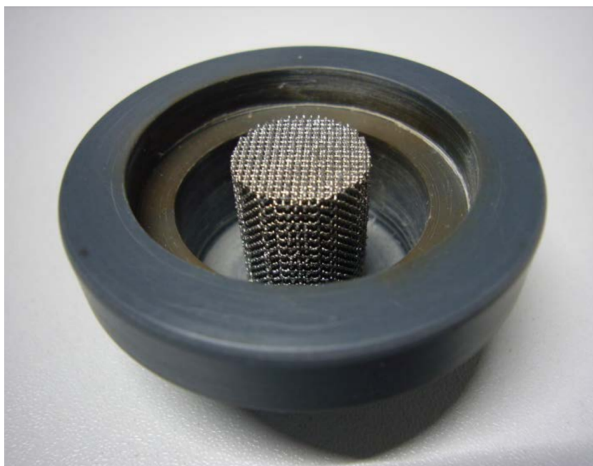
Figure 4.28: Sample with holder used for XRD measurements.
