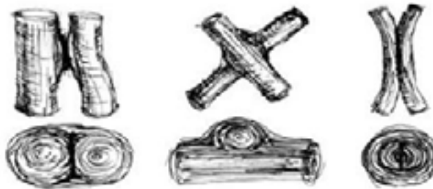
Figure 9 Typical nodes for interconnected trees: Three natural node types are studied: parallel-surface, crosswise and parallel-pith (Nuijten, 2011)
