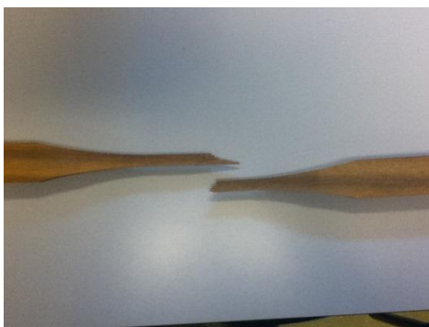
Figure 5.1. Failure pattern for a clear wood specimen of greenheart and associated load-displacement diagram under a compression test
