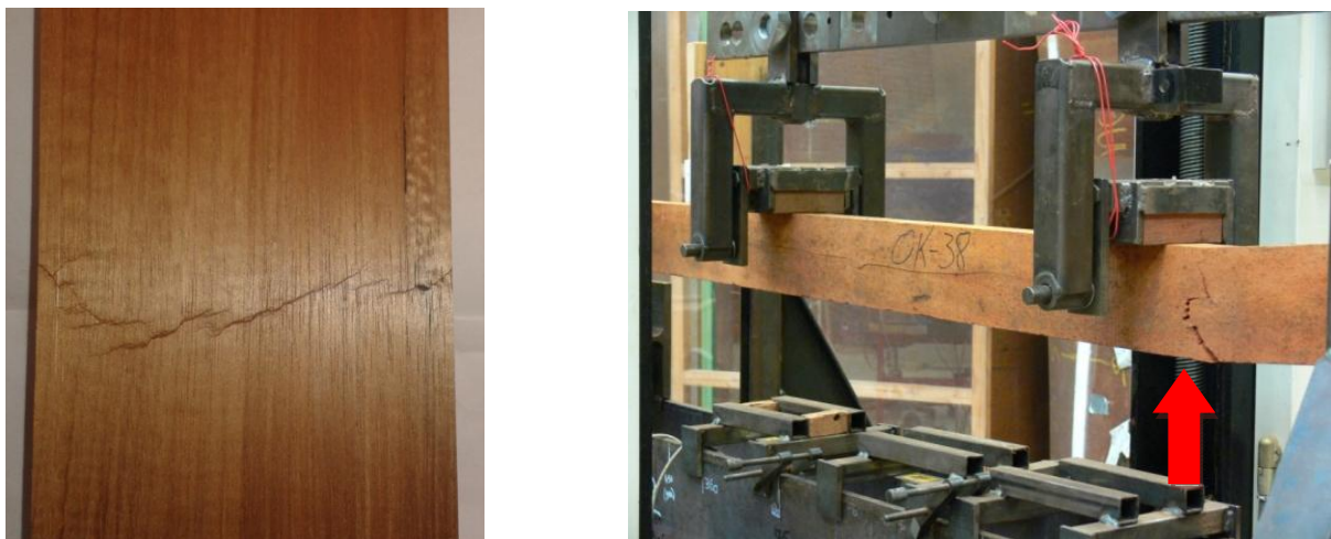
Figure 3.8. Compression failure in a timber beam (left) and the effect of a compression failure in a bending test (right).
