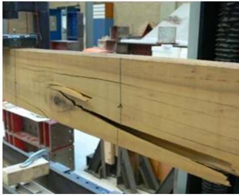
Figure 5.14b. Failure pattern for a greenheart beam with a knot and associated load-displacement diagram under a bending test.
