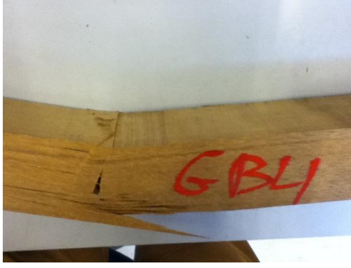
Figure 5.3. Failure pattern for a clear wood specimen of greenheart and associated load-displacement diagram under a three point bending test.
