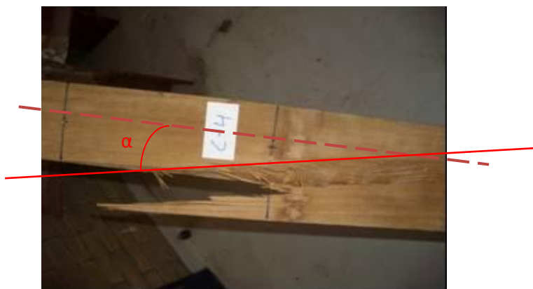
Figure 5.35. (above) Schematizing of grain angle deviation. (below) Example of grain angle deviation \alpha and failure mode in a cumaru beam tested in a four-point bending test.
