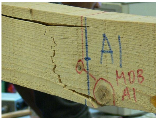
Figure 5.14a. Failure pattern for a spruce beam with knots and associated load-displacement diagram under a bending test.
