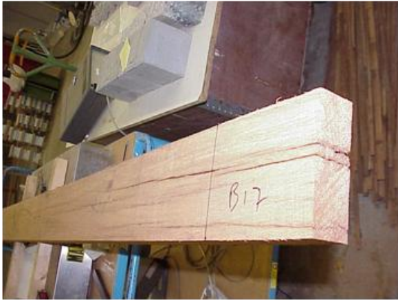
Figure 3.9. Examples of fissures that are not allowed in structural timber. On the left, an end fissure passes through the thickness. On the right, a fissure running out of the top side of the beam.
