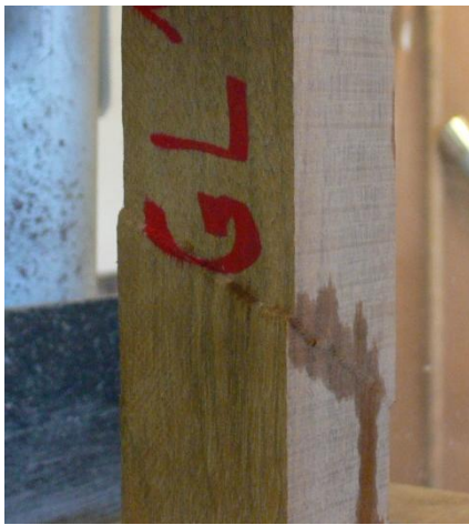
Figure 5.1. Failure pattern for a clear wood specimen of greenheart and associated load-displacement diagram under a compression test
