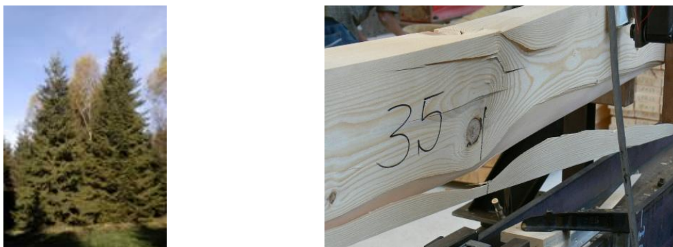
Figure 1.4. Spruce tree (picea abies) (left) and typical failure mechanism for a spruce timber beam (right)
