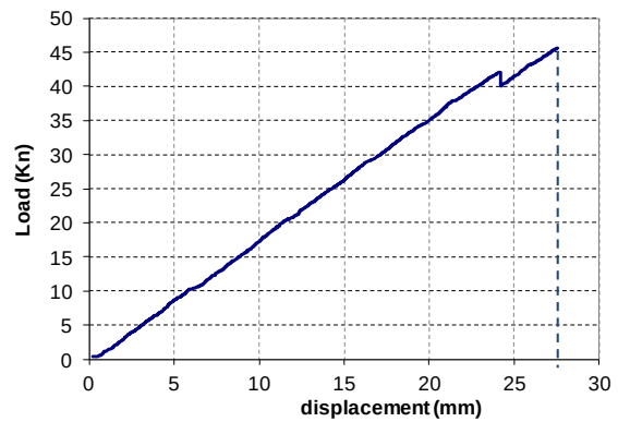
Figure 5.14b. Failure pattern for a greenheart beam with a knot and associated load-displacement diagram under a bending test.
