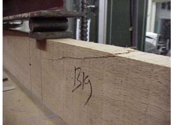
Figure 3.9. Examples of fissures that are not allowed in structural timber. On the left, an end fissure passes through the thickness. On the right, a fissure running out of the top side of the beam.
