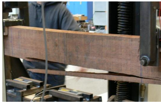
Figure 1.5. Cumaru tree (dypterix spp.) (left) and typical failure mechanism for a cumaru timber beam (right)
