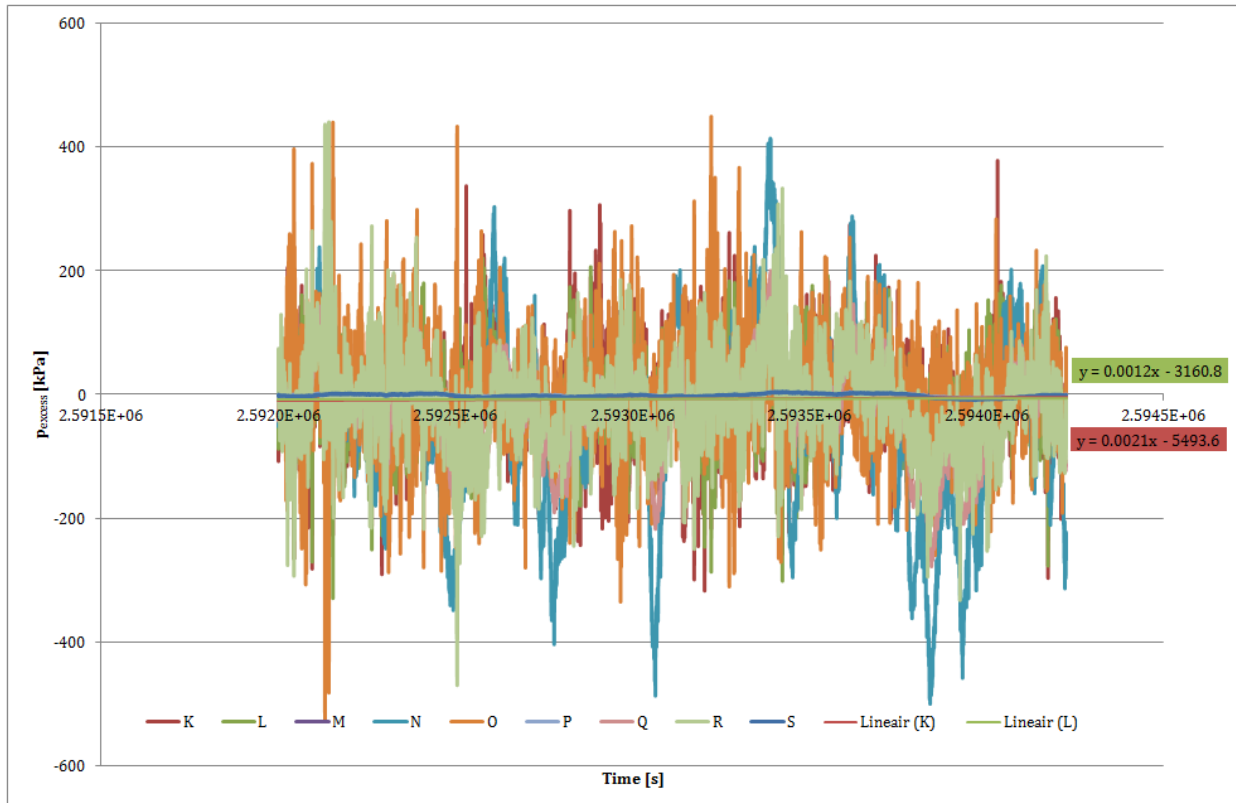
Figure 5.5: Excess pore pressure development under extreme conditions, considering the full problem geometry
