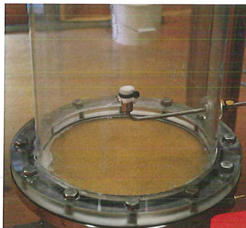
Figure 3.4: Picture of the single jet above the distribution plate inside the perspex column. The outlet of the nozzle is covered with a cloth to prevent particles from entering the nozzle when it is switched off.
