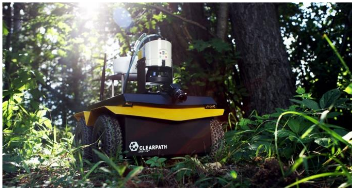
Figure 8: the autonomously driving robot 'the Jackal' (from CLEARPATH) which can be driven manually and is used in our case study to encounter participants.
