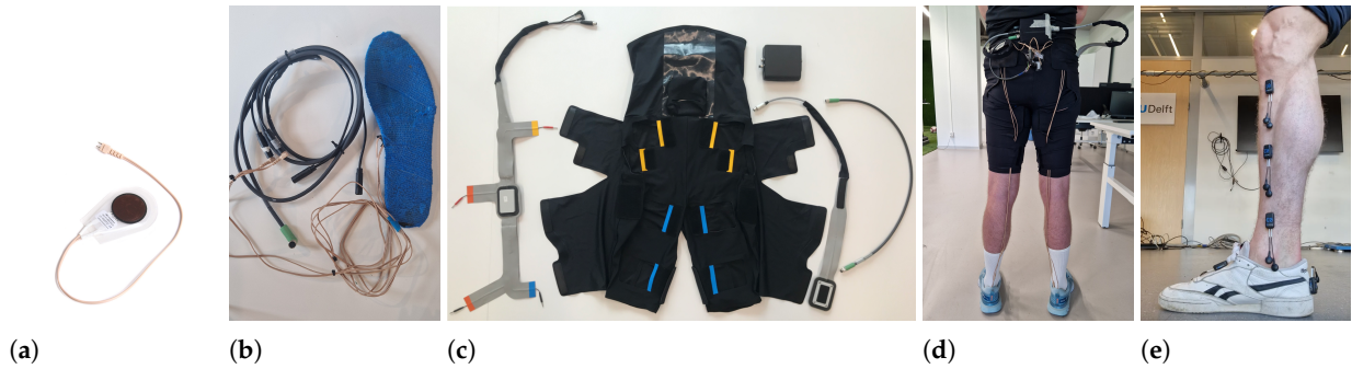
Figure 2. (a) A single force-sensitive resistor (FSR; Odstock Medical). (b) Insole footswitch system with two embedded FSRs and connecting cables. (c) Biostim shorts with control unit and thigh IMUs. (d) Participant wearing the Biostim shorts, with visible footswitch cables. (e) IMU placements on the shin and shoe.
