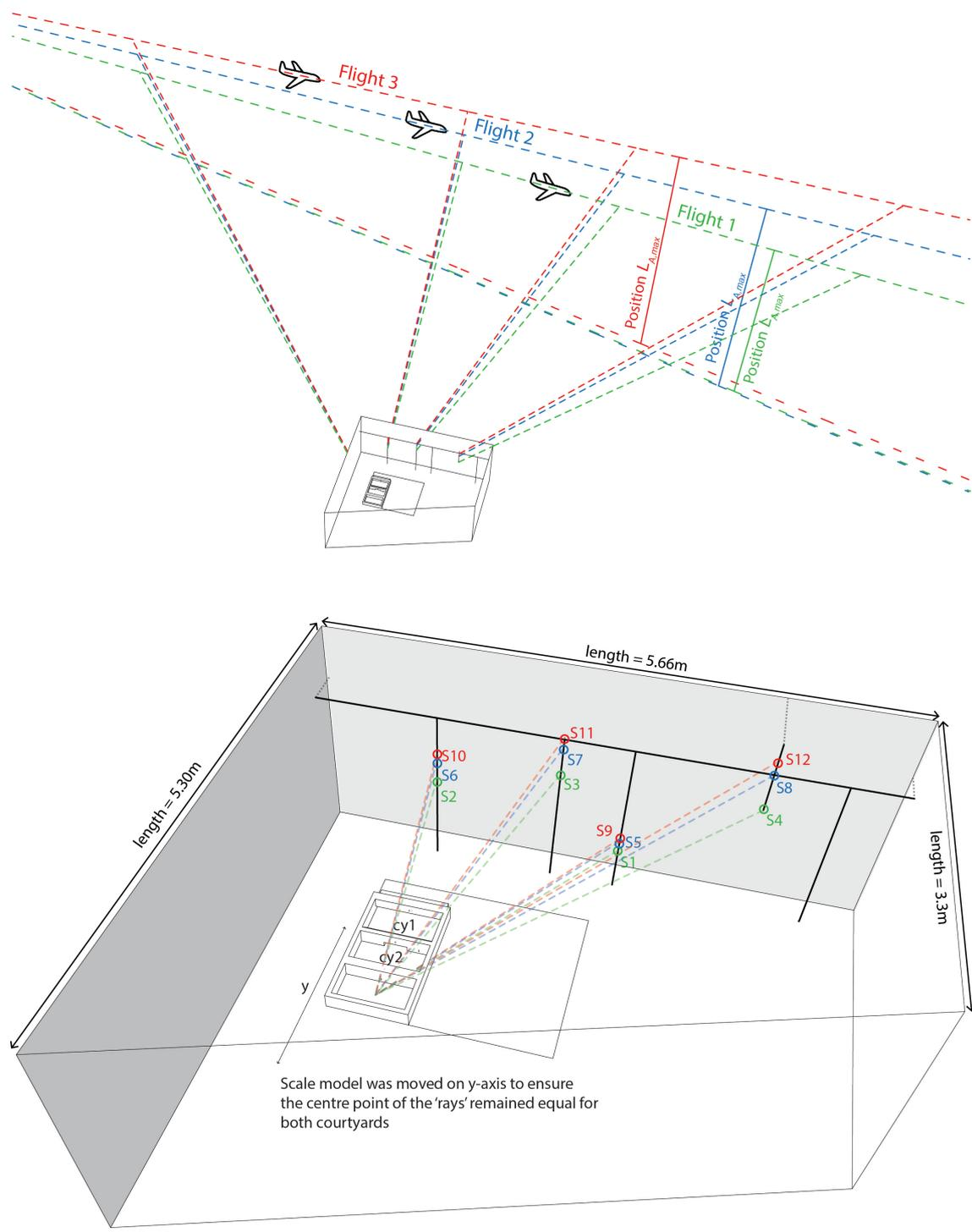
**Figure 3** (top) Flight paths relative to the field lab, the dotted lines are straight rays between the centre of the third courtyard and the x,y,z position of the stills in **Figure 2**. (bottom) Position of the speakers inside the anechoic room, cy = courtyard.
