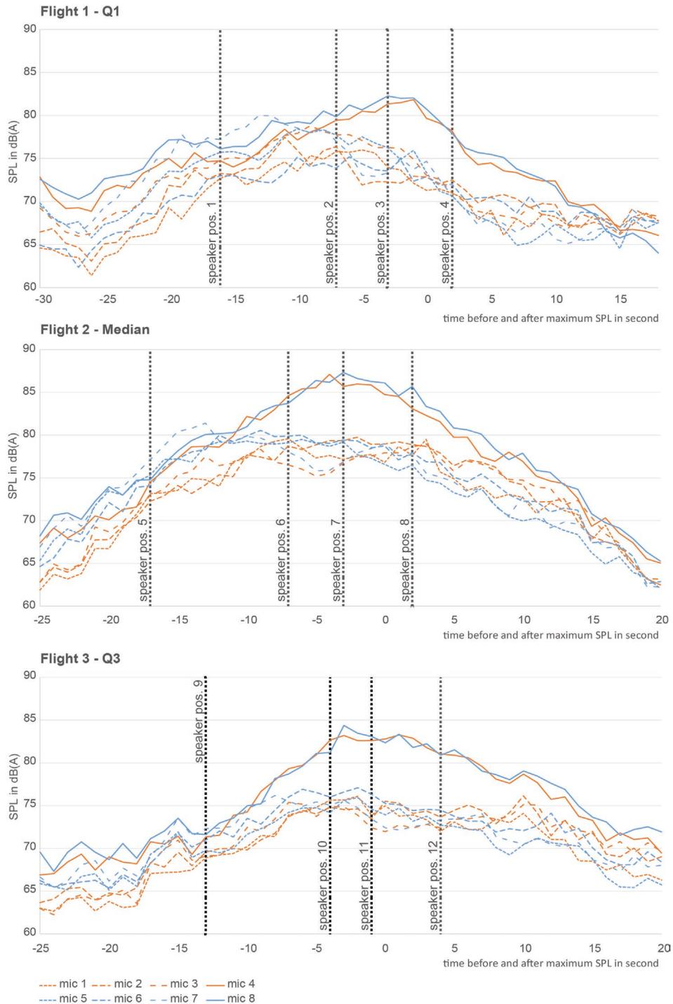
**Figure 2** Sound pressure levels for eight microphones and speaker positions / stills.
