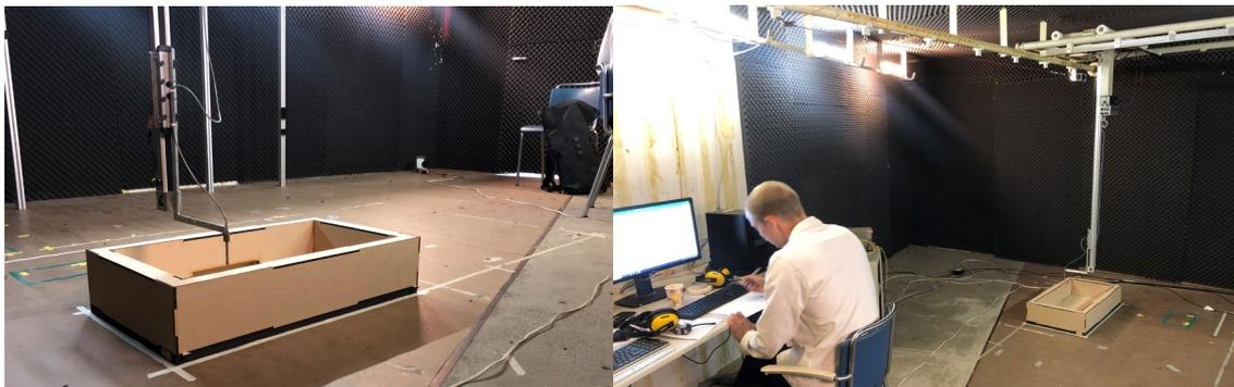
**Figure 4** Close-up of a model scale 1:50 for courtyard 2 and the microphone connected to a movable rail system (top). Scale model and the anechoic room used for the experiments (bottom).
