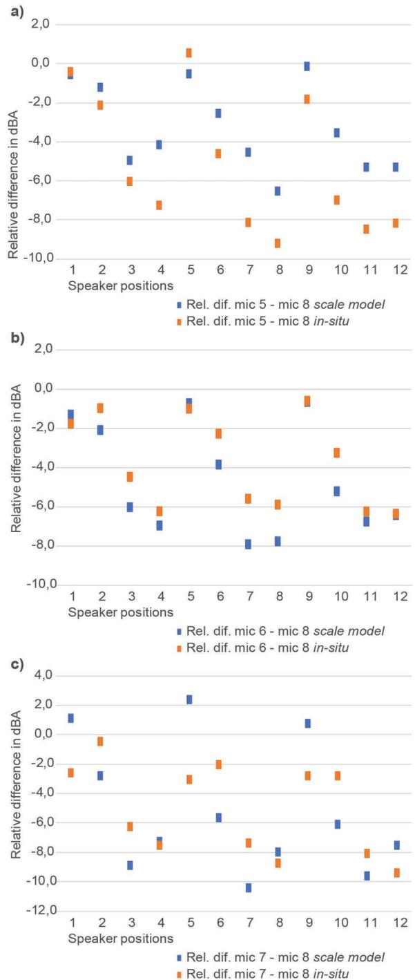
**Figure 6** Relative differences between exposed and shielded microphones for courtyard 2.
