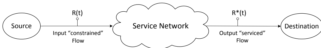
Figure 2-1: A basic network calculus model. R(t) is an arrival process and R^*(t) is a departure process.
