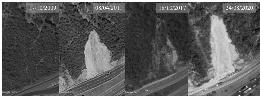
Fig. 3. Time-line showing the development of the studied landslide starting from left to right: October 2009, April 2011, October 2017, and August 2020.
