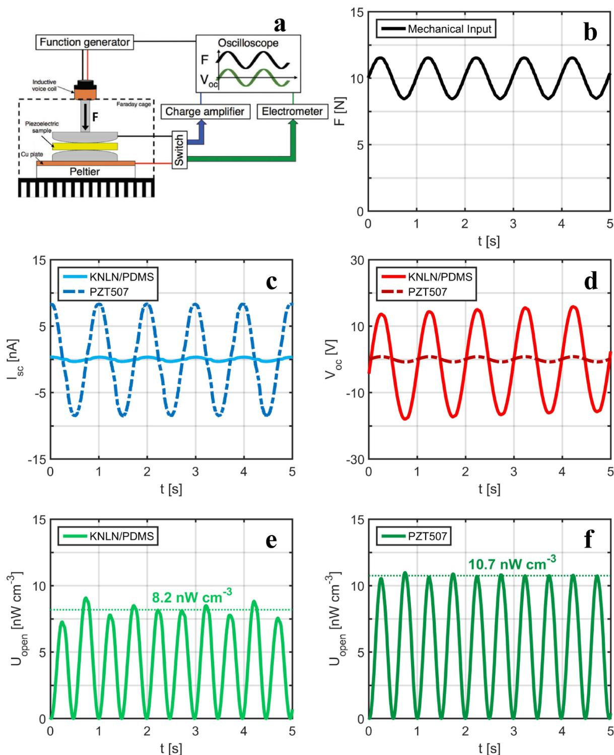
**Figure 5.** Electrical response to a mechanical input of KNLN/PDMS and PZT507, both having a thickness of 1 mm and an area of 50 mm<sup>2</sup>, measured using a specifically designed piezometer system. a) Schematic representation of the piezometer system,<sup>[10]</sup> b) the mechanical input,  $F$ , c) the short circuit current,  $I_{sc}$ , d) the open circuit voltage,  $V_{oc}$ , and the stored electrical energy,  $U_{open}$ , of e) KNLN/PDMS and f) PZT507, respectively.
