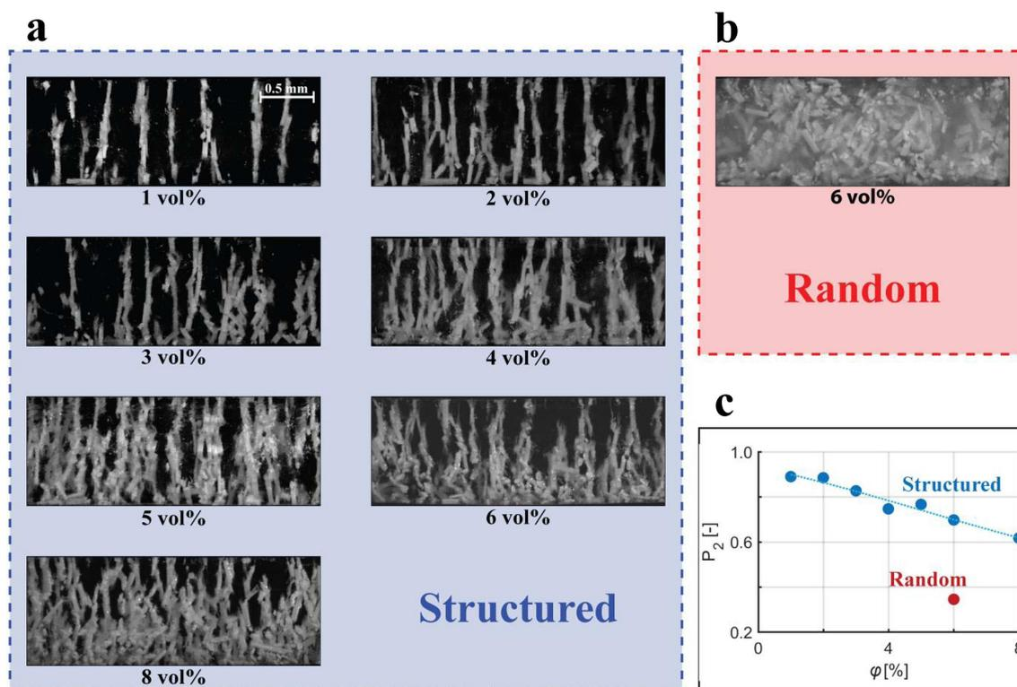
**Figure 3.** Microstructure of dielectrophoretically aligned KNLN fibers in a PDMS matrix. a) Optical micrographs of cross sections of structured composites as a function of volume fraction. b) Optical micrograph of the cross section of a random composite. c) Orientational order parameter,  $\overline{P_2}$ , as a function of volume fraction,  $\phi$ . The dotted line is a guide for the eye.
