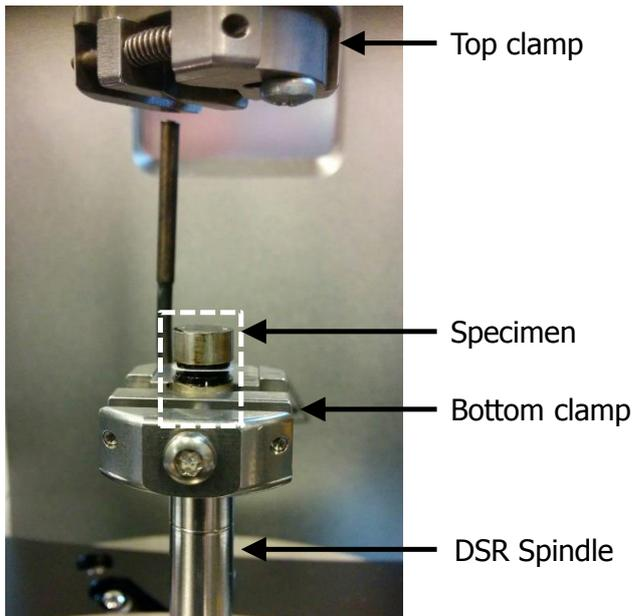
Figure 7. Specimen that has been assembled in the storage room, mounted for testing in the DSR.
