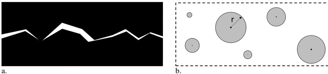
Figure 1 a. Side view of immingering contact points between two surfaces approaching. b. Top view of increasing contact area; area in contact is shown in grey, nucleating from the center point and growing radially indicated by the arrow (r).
