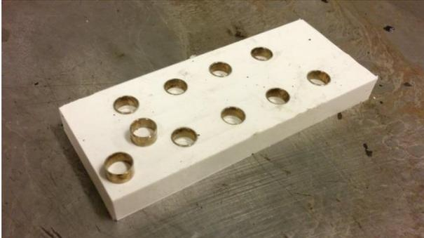
Figure 4. Silicon mold, with stainless steel rings in place during preparation of bitumen specimens.
