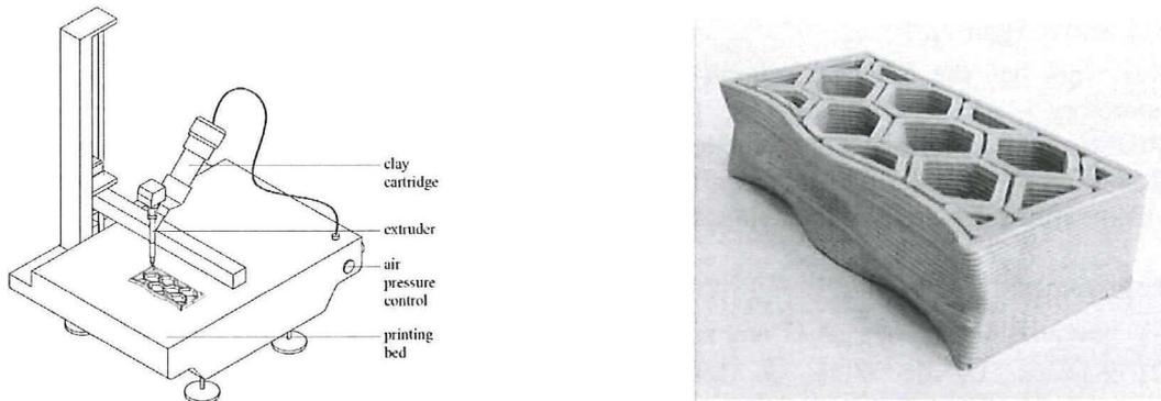
Figure 9: Lutum® 3D clay printer schema and a printed free-form stoneware brick with hexagonal inner structure
