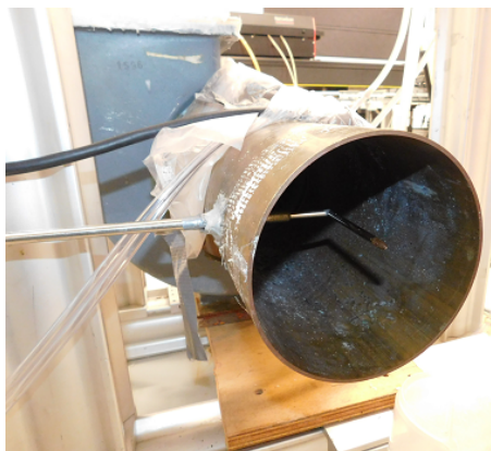
Figure 3.3: Pitot tube at the inlet of the centrifugal fan.
