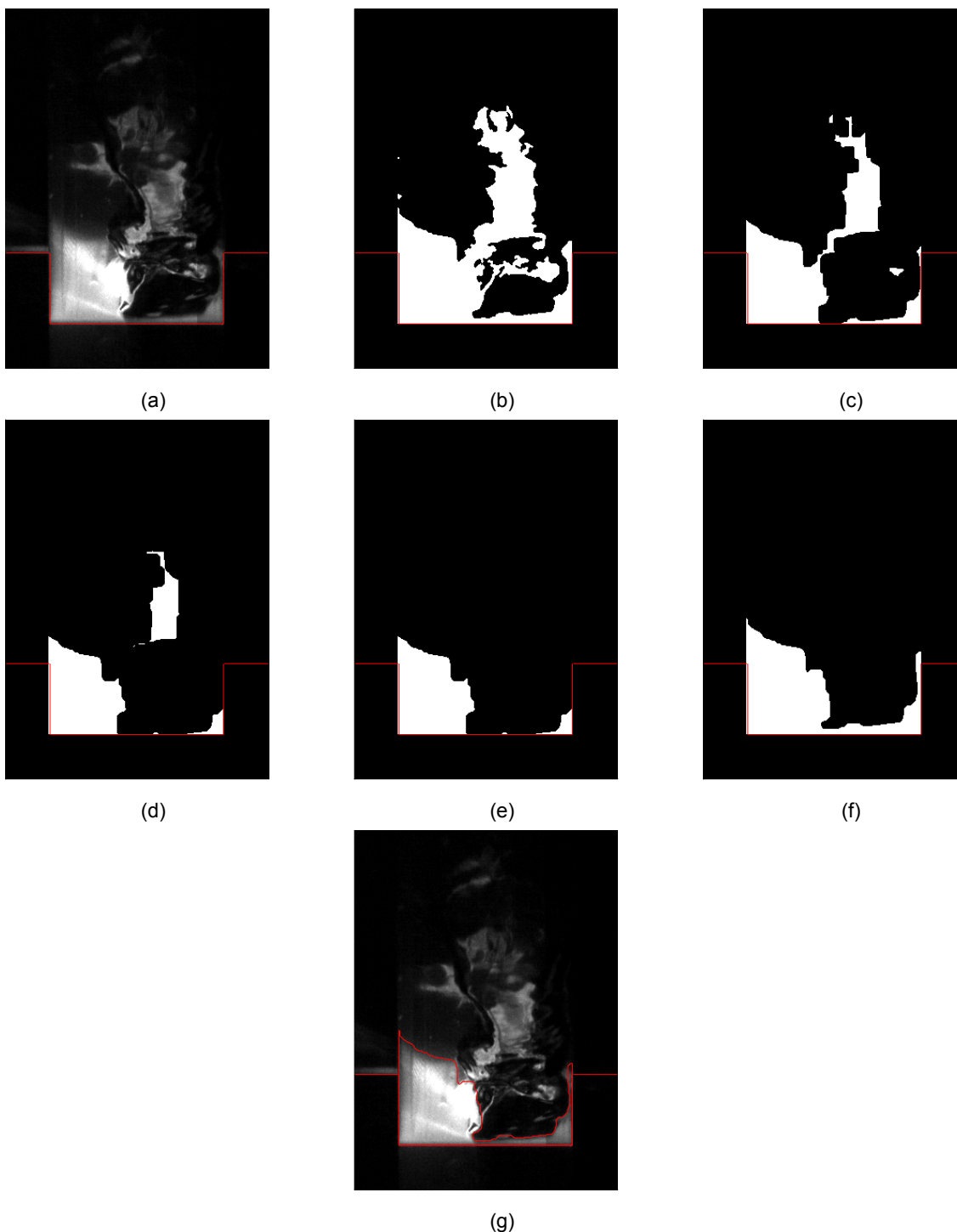
Figure 3.13: Post processing steps implemented to detect the cavity filling. (a) Raw image, (b) binarized image after applying median filter and contrast stretching to raw image, (c) erosion with first structuring element, (d) erosion with second structuring element, (e) the disjoined parts are removed, (f) dilation of the previous image, (g) the boundary obtained from dilated image plotted on top of the raw image.
