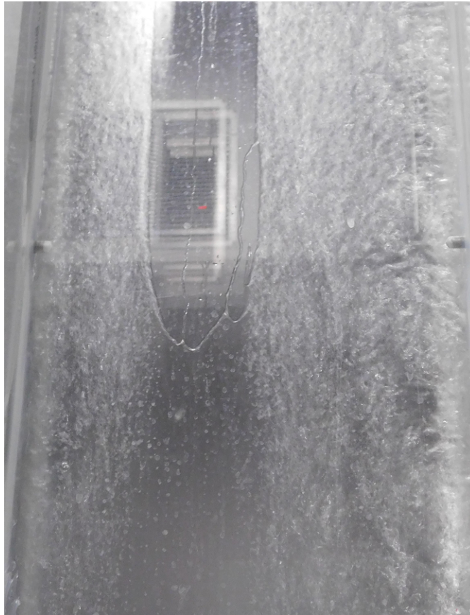
Figure 4.4: The dry patch created at the center of the channel wall.
