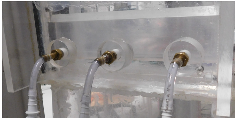
Figure 3.6: The three inlet ports of the liquid injection box.
