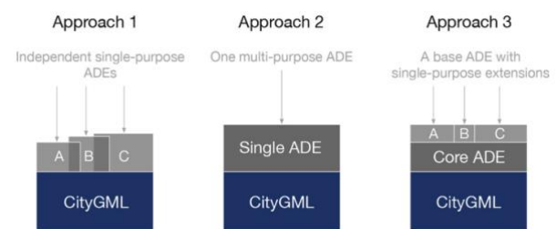
Figure 2. Different Approaches to Design an ADE for a specific or multiple use case application derived from (Biljecki et al., 2021b).
