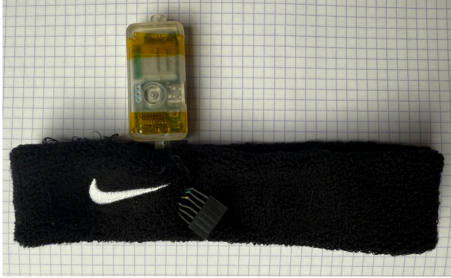
Figure 2.1: Main unit with connector for interchangeable earbud integrated into wearable head-band (developed by Dopple).
