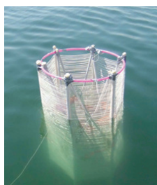
Figure 2. DTS measurement setup used in (A) Delft, and (B) Kinneret and Binaba.
