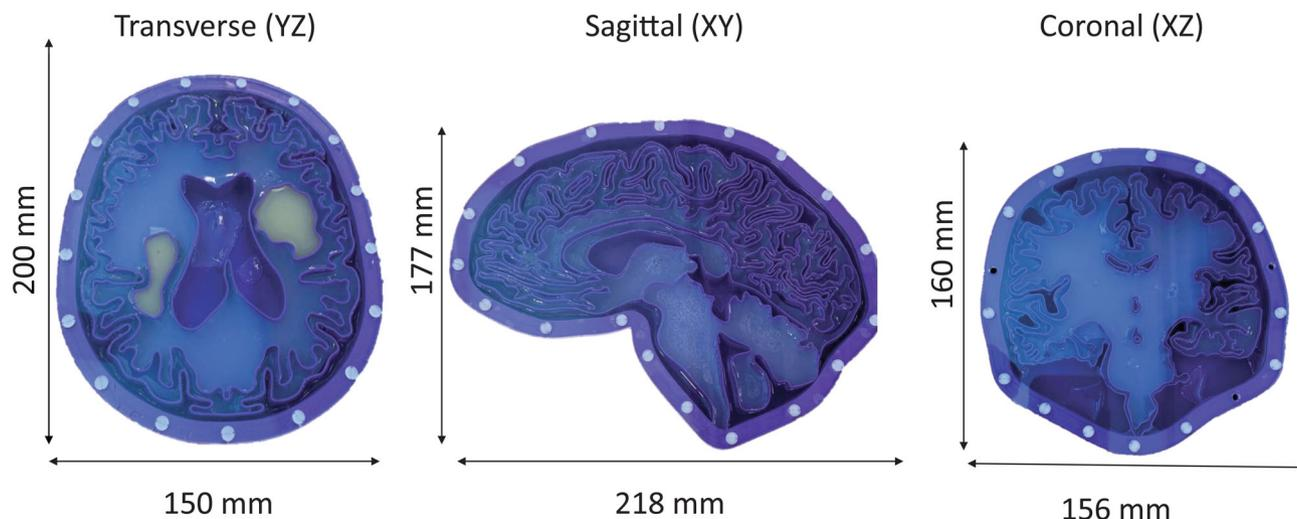
**FIGURE 2** Two-dimensional brain phantoms corresponding to transverse, sagittal and coronal brain slabs. With relaxation parameters of the compartments approximately equal to in vivo data at 50 mT.<sup>31</sup> The dimensions are indicated in the figure and the thickness of the slabs are 20 mm. The phantoms were fabricated in-house using a three-dimensional printer and modeled using CAD software and 3T brain images.
