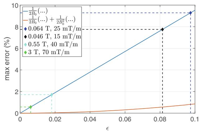
**FIGURE 9** Maximum error made using the Taylor expansion to approximate  $|\mathbf{B}|$  against values of  $\epsilon$ , different systems are indicated in the figure. Blue shows the error when only considering the  $\frac{1}{2B_0}$  terms, red when also considering the  $\frac{1}{2B_0^2}$  terms.
