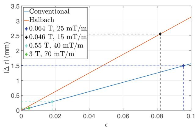
**FIGURE 8** Maximum displacement created by cross-term warping within a 250 mm DSV as a function of  $\epsilon$ . The red curve indicates warping corresponding to a Halbach-based systems while the blue curve corresponds to conventional systems. In the figure different systems and their corresponding maximum warping are indicated.
