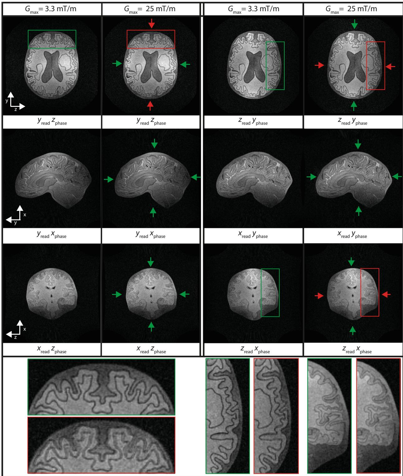
**FIGURE 5** Phantom images obtained with the two-dimensional SE sequence shown in 3(A,C), used to show the self-squared term effects. Blurring is visible in certain orientations at the outer regions of the phantoms. red arrows show where blurring is expected, green where no distortions should occur according to Equation 6. Acq param: FOV: 280x280 mm, Data Matrix: 280x280, TR/TE = 900/65 ms, BW = 40 KHz,  $\tau_d = 21$  ms, NA = 6.
