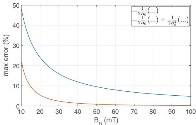
**FIGURE 10** Maximum error made using the Taylor expansion to approximate  $|\mathbf{B}|$  against values of  $B_0$ . A 250 mm field of view and constant gradient of 20 mT/m are considered. Blue shows the error when only considering the  $\frac{1}{2B_0}$  terms, red when also considering the  $\frac{1}{2B_0^2}$  terms.
