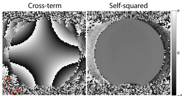
**FIGURE 7** Phase measurements of a stationary phantom using anti-symmetric bipolar pulses of 5 ms with a gradient strength of 5 mT/m. The left figure shows the phase introduced by concomitant field cross-term when playing the bipolar pulse simultaneously with the readout dephasing. In the right figure the same sequence is used but with the gradient lobes applied sequentially.
