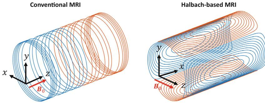
**FIGURE 1** Left: illustration of a typical wire pattern for a  $z$ -gradient coil used in conventional MRI systems. Right: illustration of a typical  $z$ -gradient coil used in Halbach-based MRI systems. Corresponding coordinate systems are displayed with each gradient coil.
