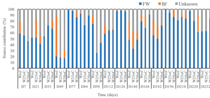
Figure 3.8: The results of source tracker method, showing percent contributions of microbial communities from different sources (feed water =FW, biofilm from relevant pilot DS=Bf, Unknown sources) into sinks ( W_{ref} = water from reference system, W_{25^{\circ}C} = water after cold recovery ( T_{max} = 25^{\circ}C ), W_{30^{\circ}C} = water after cold recovery ( T_{max} = 30^{\circ}C )) on each water sampling day.
