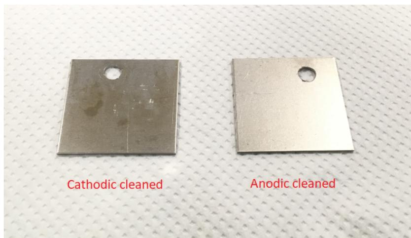
**Figure 4.7:** Discolouration of a cathodic cleaned DP800 compared to an anodic cleaned DP800 sample
