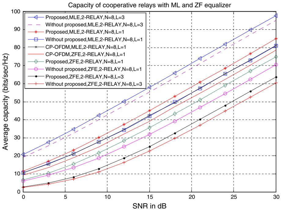
**Fig. 8** Average capacity of cooperative ZP-OFDM with ML and ZF equalizer
