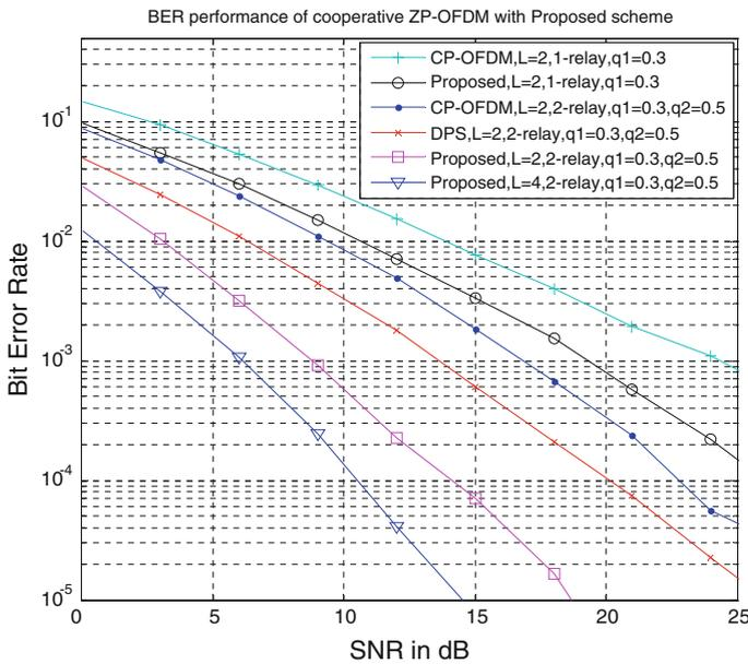
**Fig. 6** Comparison of the proposed scheme to other conventional schemes for full diversity with LEs and CFOs
