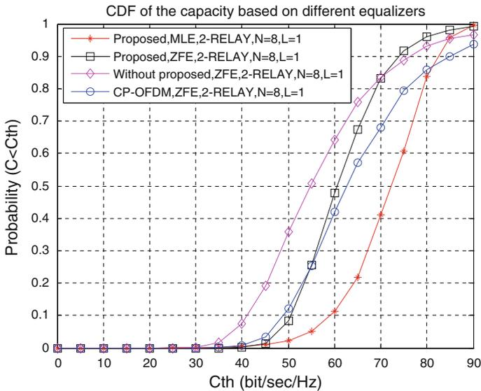
**Fig. 9** CDF of the capacity of cooperative ZP-OFDM with ML and ZF equalizer
