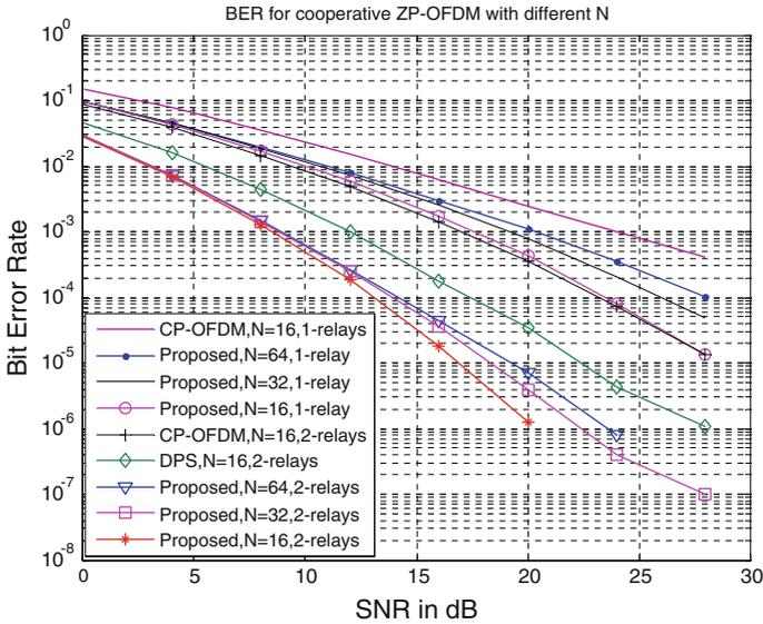
**Fig. 7** Comparison of the proposed scheme with different numbers of sub-carriers and relays
