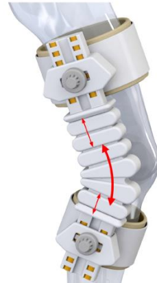
Skewed rotary elastic chambers bending actuator
