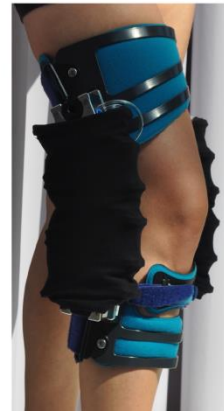
Skewed rotary elastic chambers bending actuator
