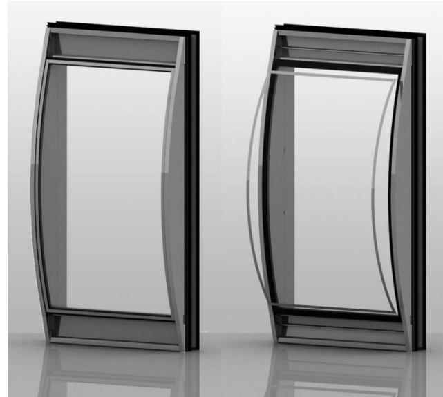
Water and air tight bending facade Source: (Özhan, 2017)
