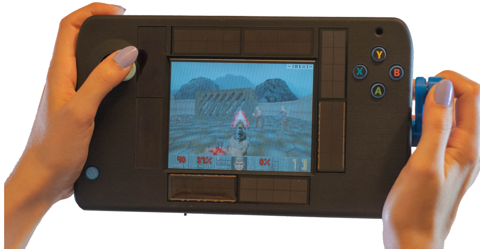
Figure 1: The battery-free TURNER console in action. Turning the crank enables weapon firing in the game DOOM, whilst at the same time generating energy to charge TURNER’s energy storage capacitor. The charging state of the capacitor is displayed by a small indicator at the top right hand side of the Liquid Crystal Display (LCD) panel. TURNER integrates solar energy harvesting sources, follows the form-factor of a modern handheld games console, and has the typical “ABXY” button configuration of a game controller. As implemented, TURNER weighs 509 g, its casing dimensions are 24 cm x 14 cm x 3 cm, and crank dimensions are 2 cm x 6.5 cm x 2 cm.
