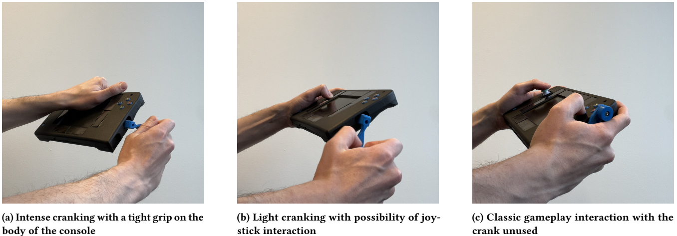
Figure 5: Example frequent console interactions during gameplay sessions. We observed that console-chassis holding techniques varied according to the intended user interaction, which itself was shaped by the energy and game input configuration of TURNER.
