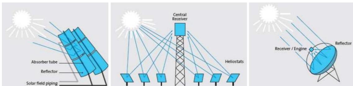
**Figure 1.** Representation of the different types of CSP plant. From left to right: parabolic trough, solar tower and dish system. Retrieved from Koroneos et al. (2008).
