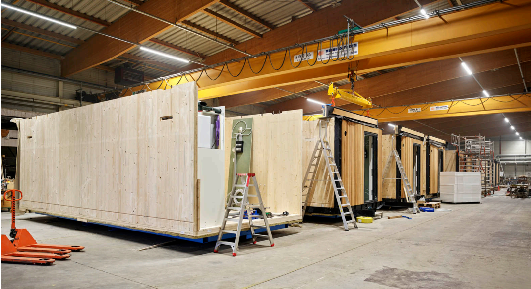
Figure 3: Factory for 3D CLT modules in Vroomshoop, The Netherlands (Source: De Groot Vroomshoop)
