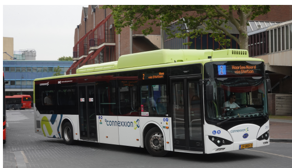
Figure 2.1: A BYD-brand in-wheel driven BEB
