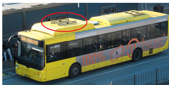
Figure 2.6: A BEB equipped with bus-down charging rail [37]
