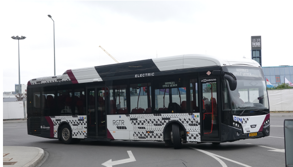
Figure 3.4: A Low-entry utility BEB
