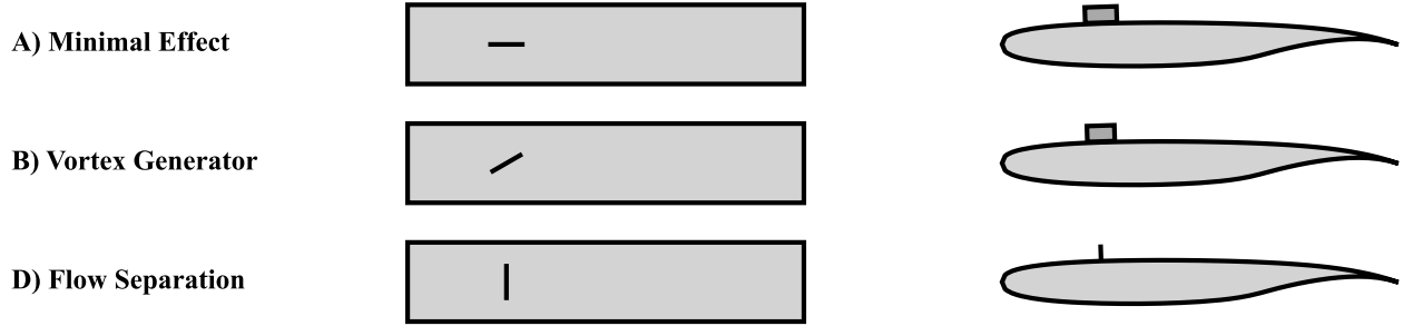
Fig. 1 Concept design of a switchable vortex generator: (A) position of minimum impact on drag for nominal cruise conditions; (B) vortex generation to suppress/delay separation at high angles of attack and low speeds; (C) spoiler configuration causing massive airflow separation for gust load alleviation.
