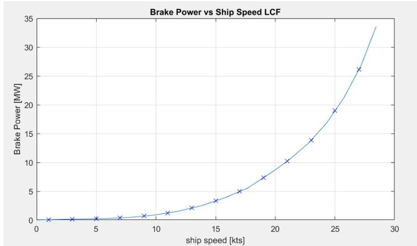
Figure 2.1: LCF Estimated brake power
