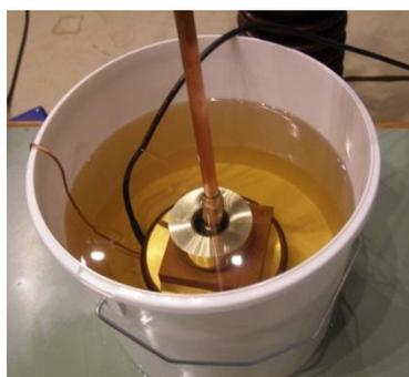
Figure 35: Sample to be tested placed between the electrodes for tan $\delta$  measurements.
