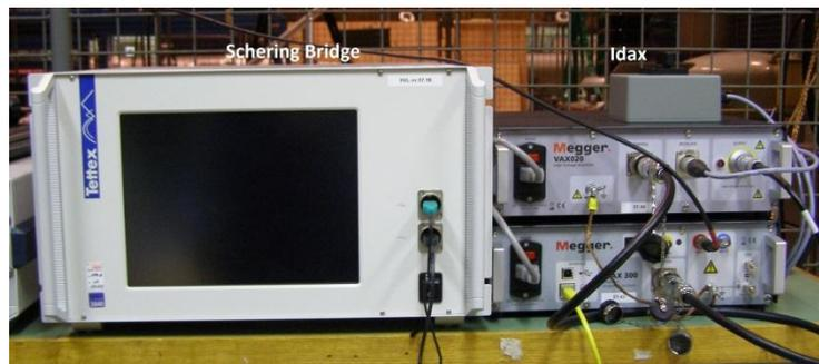
Figure 38: LV side; TETTEX and IDAX for measuring  $\tan\delta$
