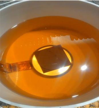
**Figure 40: Prepared container for PD measurement: Impregnated sample on the top of LV electrode**
