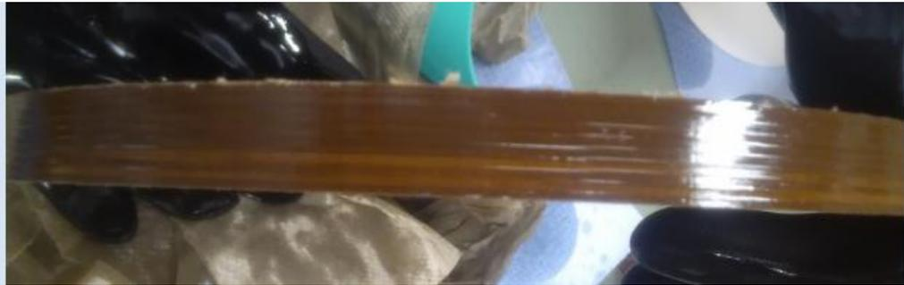
Figure 63: Sample Type III with not permeable side area to oil
