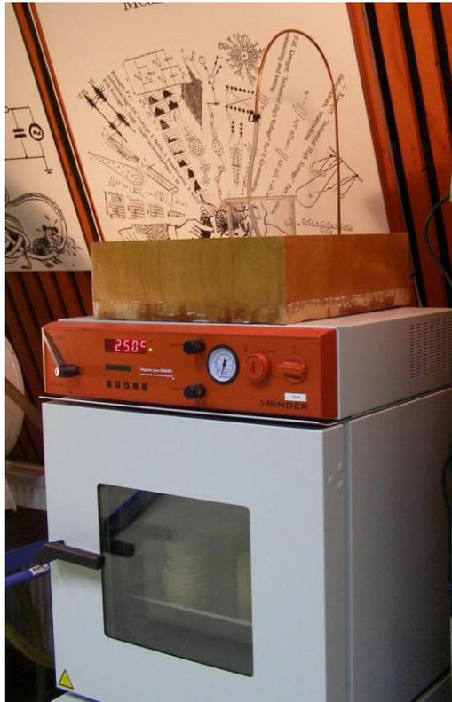
**Figure 26: Vacuum oven used for Impregnation**
