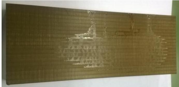
**Figure 64: Sample with glue leaking on the side surface**
