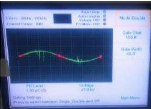
Figure 44: PD activity observed during testing of sample type a)
