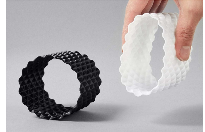
Figure 7.7- Flexibility of TPU made with FDM (3D people, n.d.)
