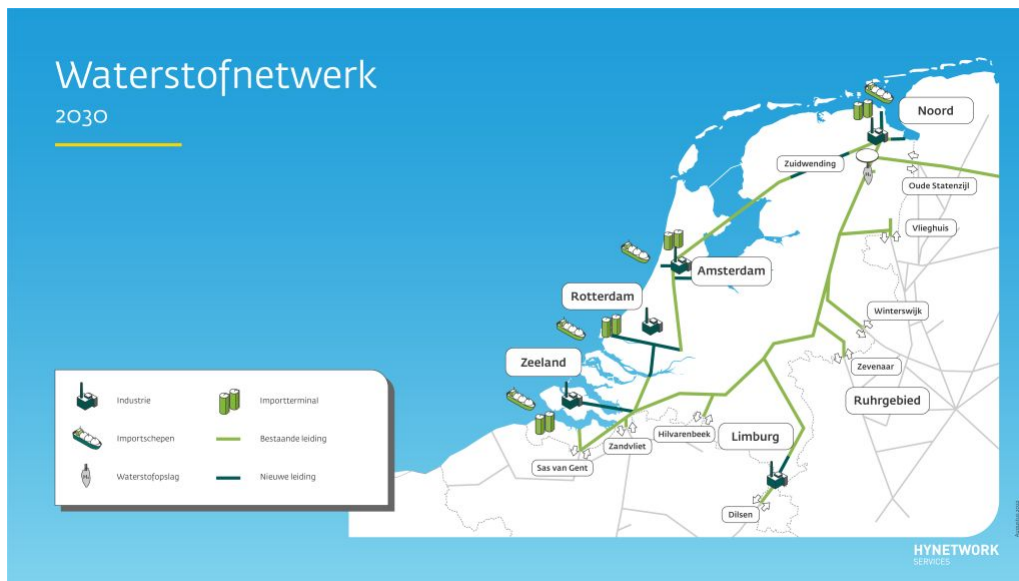
Figure 1.4: 2030 Hydrogen Network by Gasunie [15]
