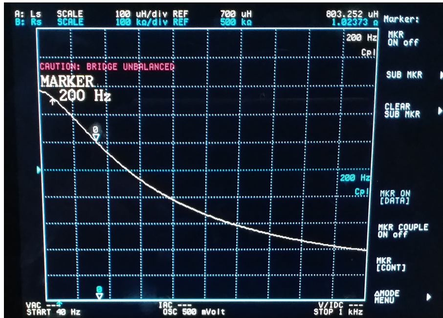
Figure 2.5: Self-inductance measurement for one winding from impedance analyzer.
