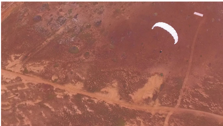
Fig. 7.1 Airborne wind energy system with 60 m 2 kite and suspended robotic control unit, operating on the Caribbean island Aruba in October 2021. Video still of the original drone footage with enhanced red tones (Schmehl 2022). Courtesy of Kitepower B.V.
